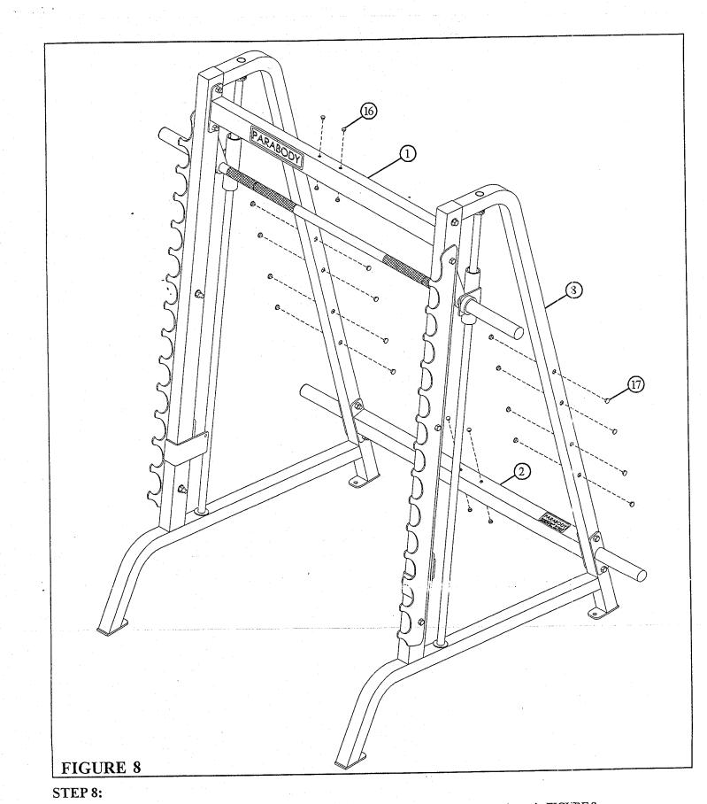
• Insert sixteen 9/16" CAP PLUGS (17) into the exposed holes in the UPRIGHT FRAMES (8) as shown in FIGURE 8.
